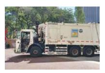
DSNY collector truck with Vision Zero-branded side guard
