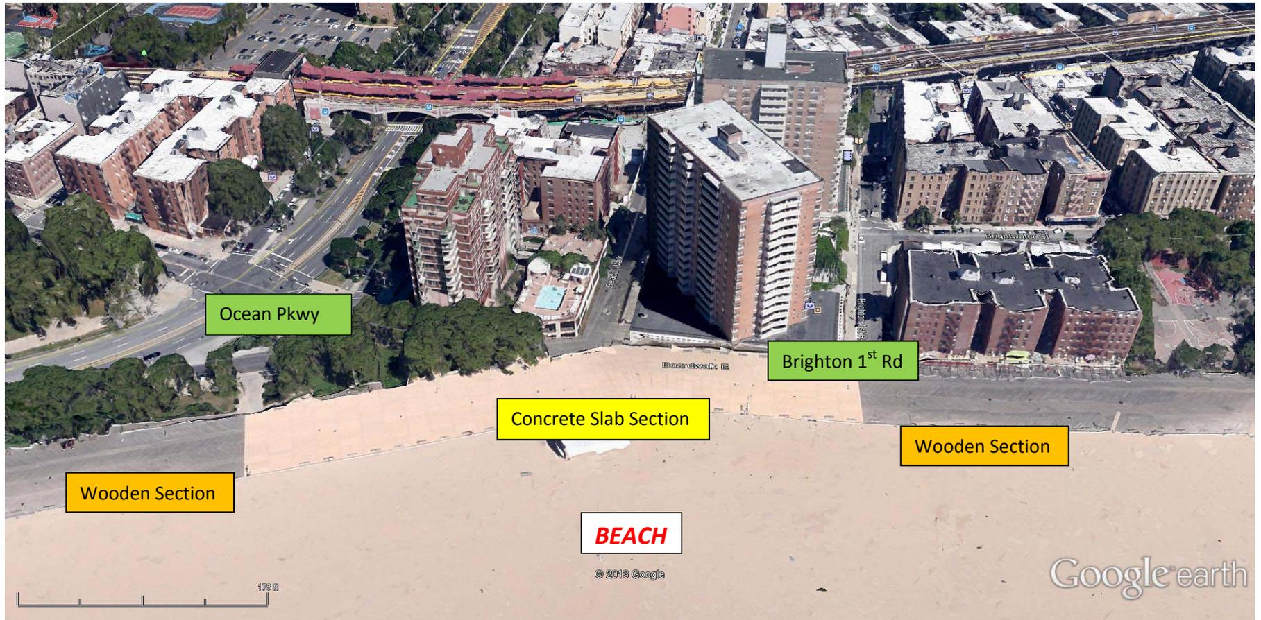
A few years ago, a section of the wooden Boardwalk (between Ocean Parkway & Brighton 1<sup>st</sup> Road) was replaced with concrete slabs, as a pilot project.
