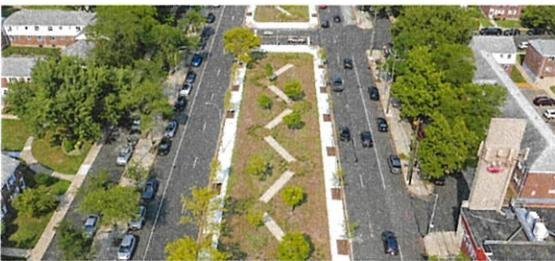
Greened medians, or Stormwater Greenstreets, are planted areas designed to collect and manage stormwater that runs off the streets and sidewalks. Unlike curbside rain gardens, these are typically constructed in the roadway, are usually larger than rain gardens, and have varying lengths, widths and soil depths based on the characteristics of the existing roadway.
