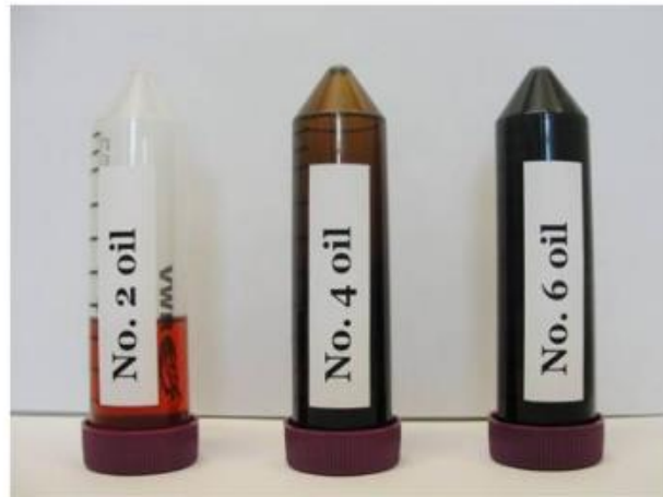
Pictured are vials of ULS 2, No. 4, and No 6 heating oil. Each vial was one third full and was shaken before photographing. Note that ULS 2 heating oil is dyed red
