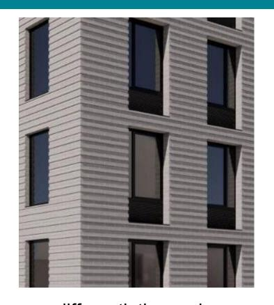
Multiple brick colors and brick articulation incorporated to provide more differentiation and movement across the facade
