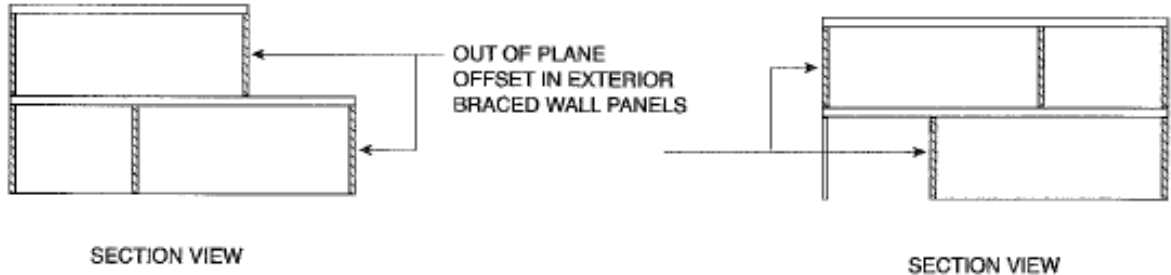
FIGURE 2308.12.6(1) BRACED WALL PANELS OUT OF PLANE
