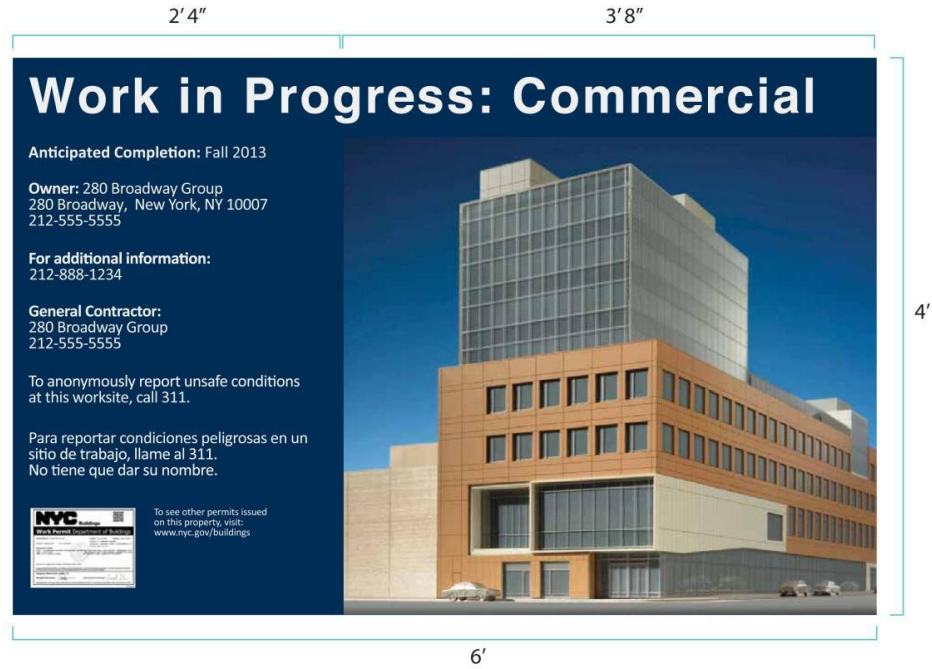
FIGURE 3301.9.1.4(2) FENCE PROJECT INFORMATION PANEL LAYOUT
