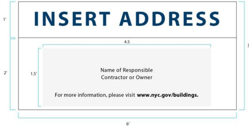
FIGURE 3301.9.2.1(1) SIDEWALK SHED PARAPET INFORMATION PANEL LAYOUT
