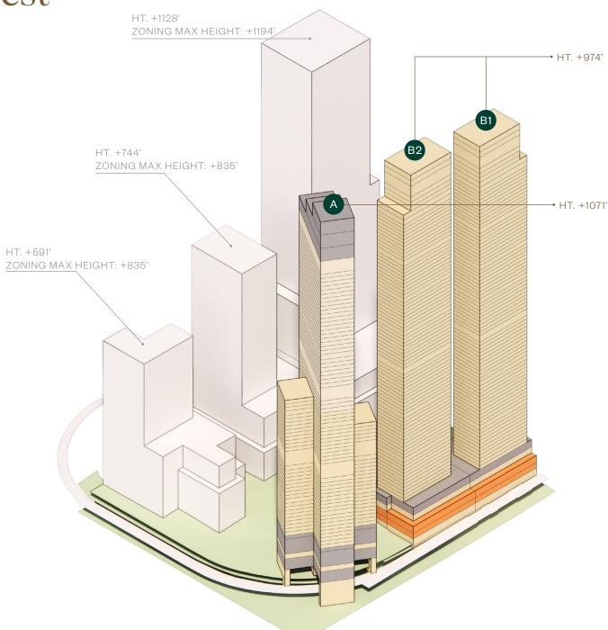
Notes: EL +00' Elevation Levels shown are based on NAVD88 elevation datum. HT +00' Building Heights are measured from Site datum at +33'8" based on NAVD88 elevation datum.
