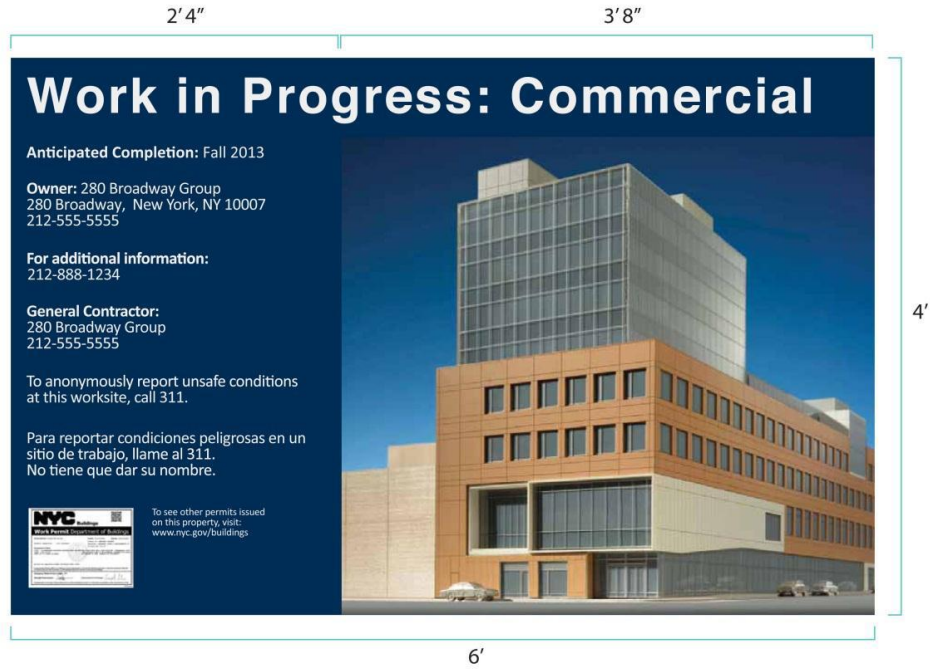
FIGURE 3301.9.1.4(2) FENCE PROJECT INFORMATION PANEL LAYOUT
