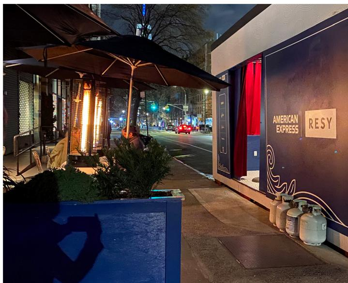
Improper propane tank storage; propane heaters too close to combustible materials
