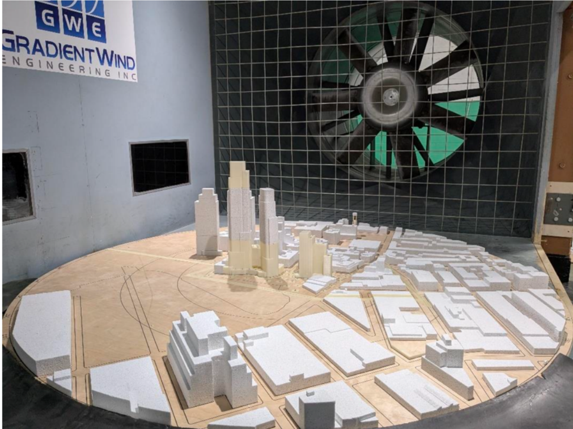
PHOTOGRAPH 1: STUDY MODEL INSIDE THE GWE WIND TUNNEL LOOKING DOWNWIND Source: DEIS, Appendix D, Wind Study
