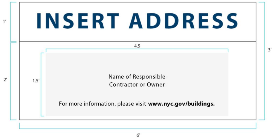
FIGURE 3301.9.2.1(1) SIDEWALK SHED PARAPET PANEL LAYOUT
