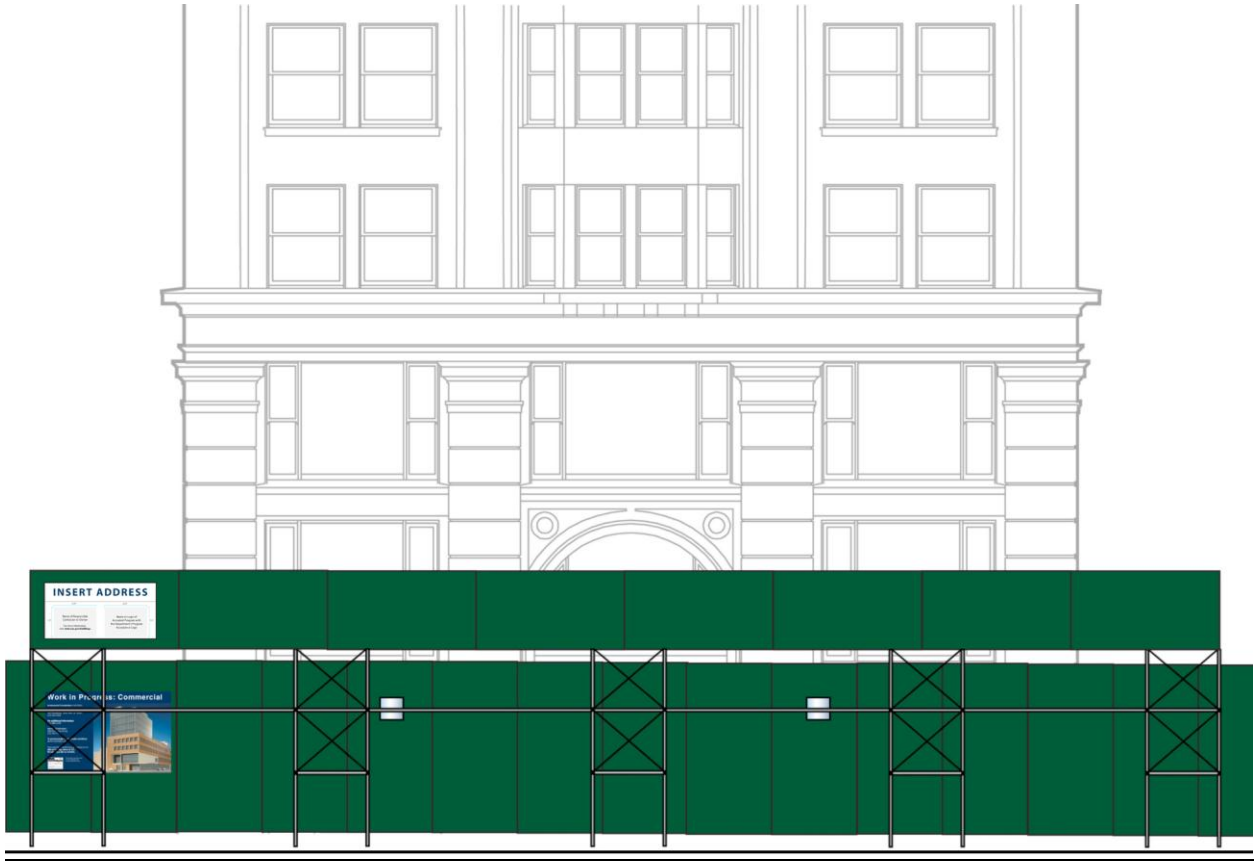
FIGURE 3301.9.2.2 PANEL POSTING ELEVATION DIAGRAM
