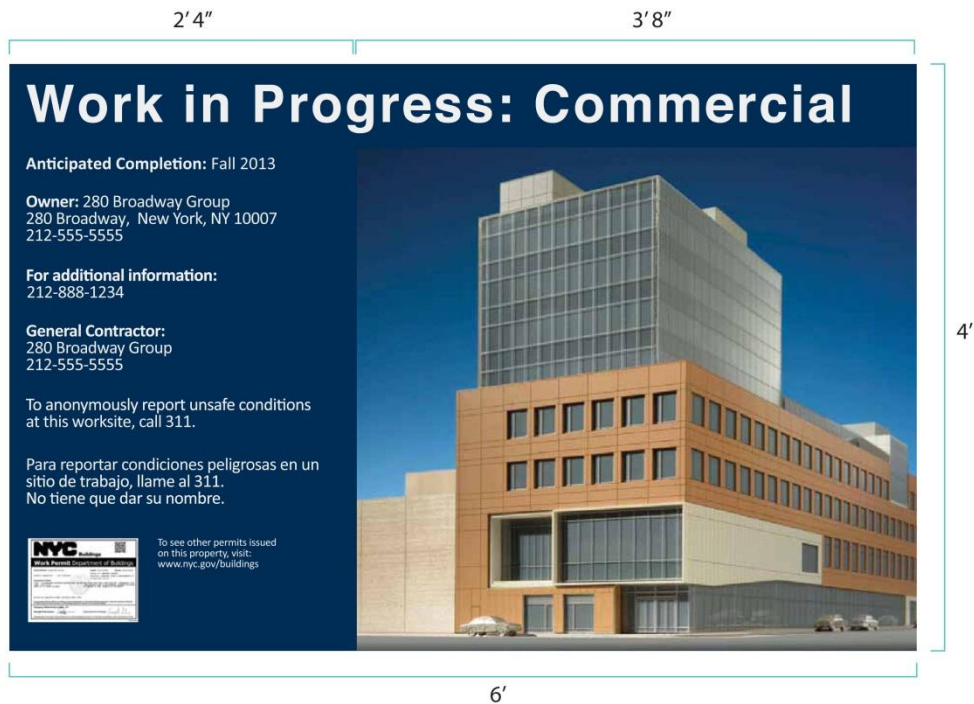
FIGURE 3301.9.1.4(2) FENCE PROJECT INFORMATION PANEL LAYOUT
